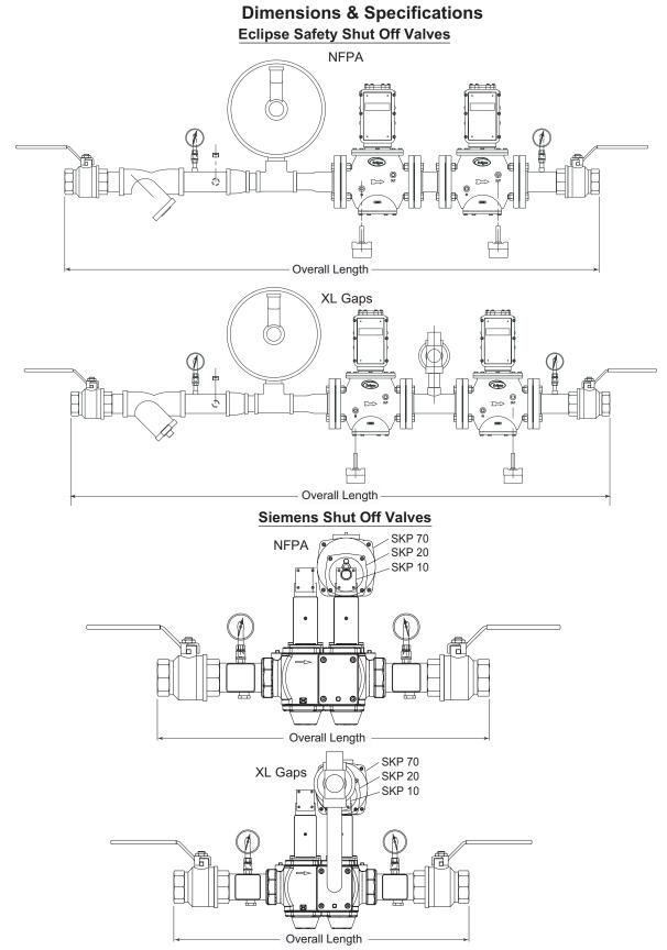
When using the Siemens SKP20 and SKP70 actuators for pressure regulating and ratio regulating functions, the sensing piping is not included. For proper operation, the sensing pipe should be at least 1/4" ID and connected a minimum of 5 pipe diameters downstream in a non-turbulent area.
